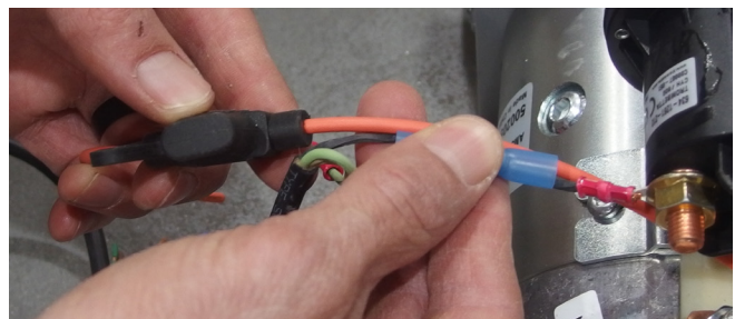
Orange fuse wire connects to the black wire and is connected to the input on the motor start solenoid.
